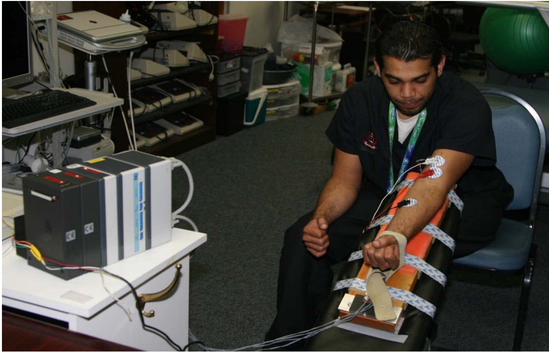
Figure 8. A typical subject exerting force on the strain gauge device.
