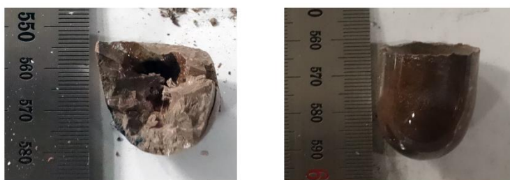
Figure 6. Optical photographs of the used salt ingots after electrorefining in (left) LiCl-KCl-ZrCl_4 (2.0 wt.%) and (right) LiCl-KCl-ZrCl_4 (4.0 wt.%)
