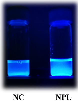
Figure 15. a) Photoluminescence of unpurified nanoplatelets. b) PL data of purified nanoplatelets and nanocubes with same emission. c) photograph showing PL of blue perovskite nanocrystal solution with different shape.
