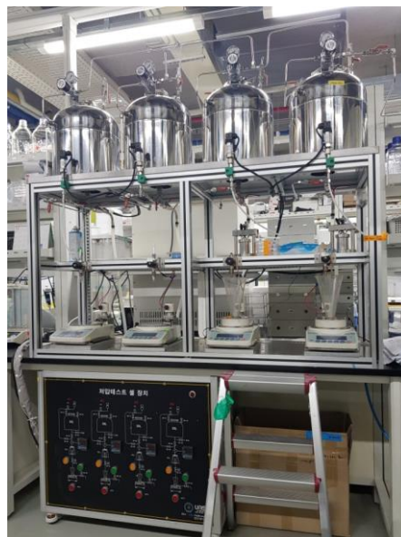
Figure 15. Dead-end filtration system
