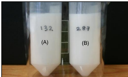
Figure 3.1 Lotion with VCO-SLPs (A) and without VCO-SLPs (B) after centrifugation
