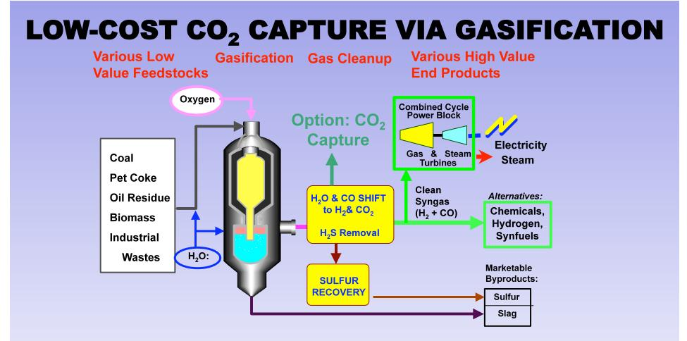
Gasification in O<sub>2</sub>/steam converts carbonaceous feedstock into syngas (mostly CO, H<sub>2</sub>)
