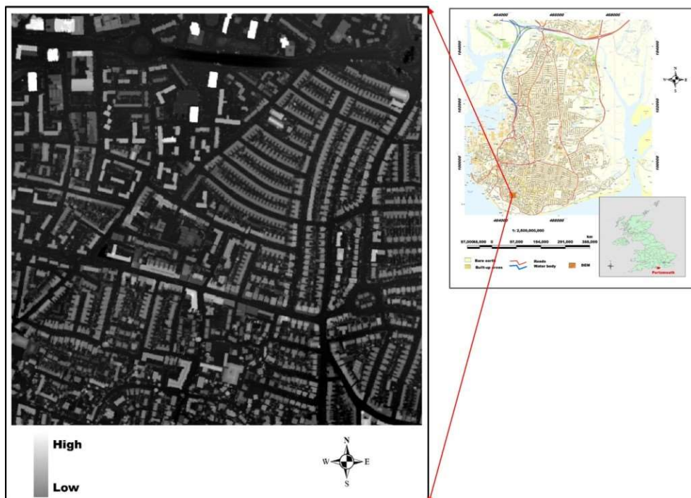
Figure 7-3: Sample of LiDAR DEM for the Portsmouth study area.
