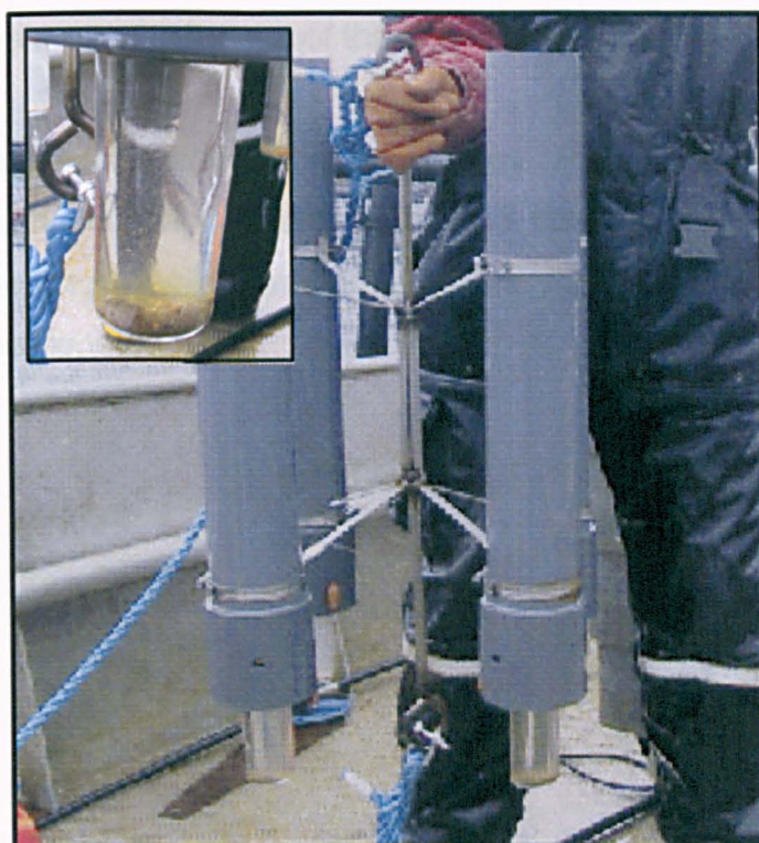
Figure 4.1 Sediment trap design used to collect particulate material around fish farms. 4-off PVC tubes of length 60cm and diameter 8cm (Aspect Ratio 7.5:1). Tubes held at 90° from each other on a central ungimballed spigot. Distance between tubes on opposing legs was 43cm. Samples accumulate in 150ml Sterilin polystyrene metal capped containers, 100ml at the reference site (inset).
