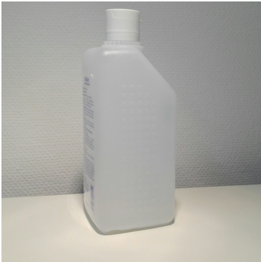
(a) The water-filled bottle used as a phantom
