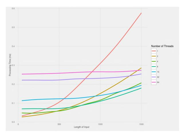
Figure 8.9: Horspool algorithm: Input processing time versus number of inputs for Dataset D.
