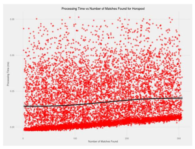
Figure 8.5: Horspool algorithm: Input processing time versus number of matches for  $Dataset \ F.$
