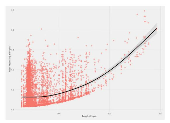
Figure 7.11: Rabin-Karp algorithm: Input processing time versus input length for Dataset A.
