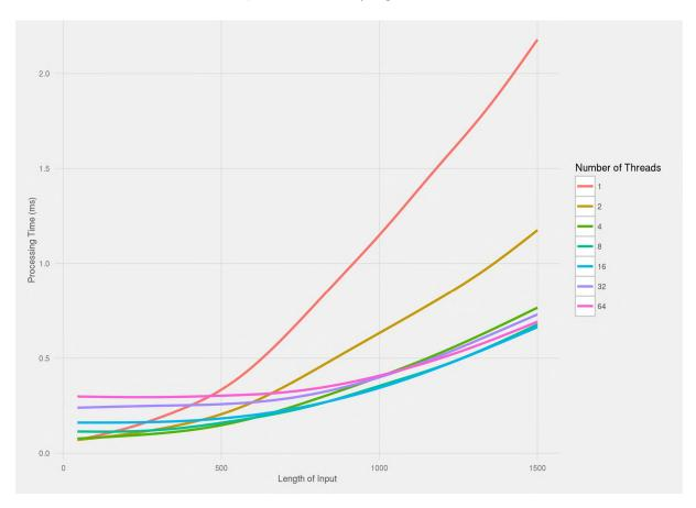
Figure 8.11: Not So Naïve algorithm: Input processing time versus number of inputs for *Dataset D*.
