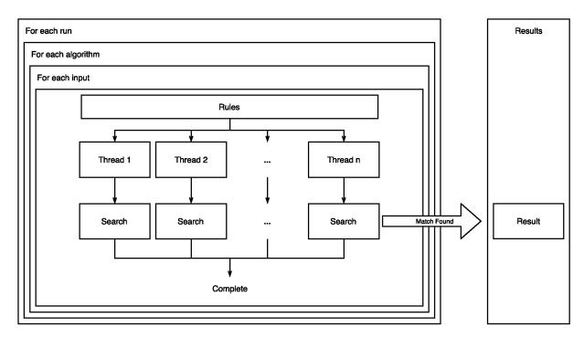
Figure 5.3: The functioning of the main processing logic of the test system.
