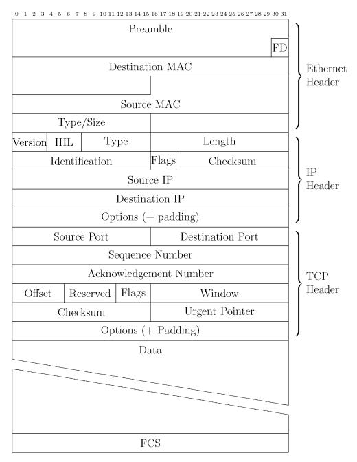
Figure 2.6: An example packet. Different levels of packet inspection have access to different protocols within a packet.
