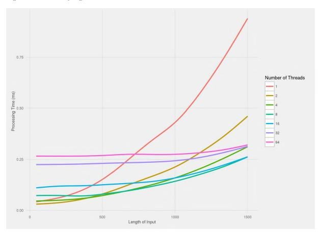
Figure 8.10: Quick Search algorithm: Input processing time versus number of inputs for Dataset D.
