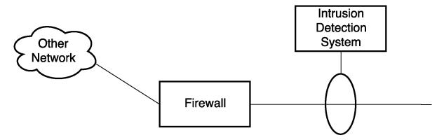
Figure 2.2: A traditional network setup with a firewall at the network edge and the Intrusion Detection System behind it.
