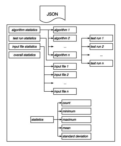
Figure 5.5: The structure of the output of the statistics generation
