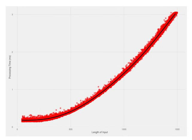
Figure 8.4: Rabin-Karp algorithm: Input processing time versus input length for Dataset C.
