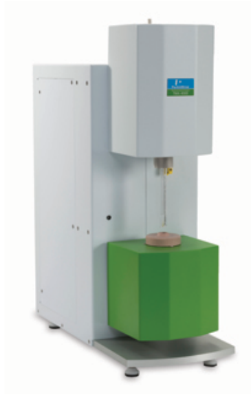
Figure 3.6: Apparatus used to determine thermal response of the material PerkinElmer TMA 4000.
