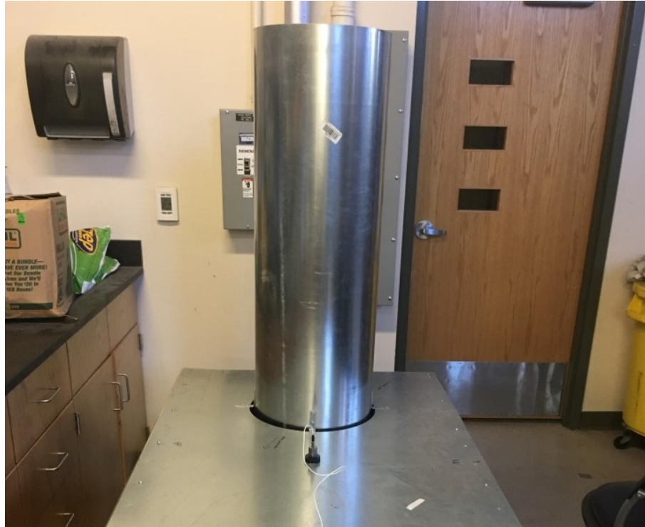
Fig. 5.12. Experimental setup to measure the free vibration of the roof.
