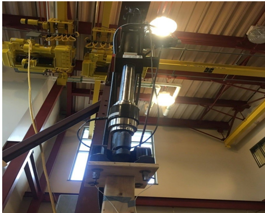
Fig. 3.3. Experimental setup with two accelerometers and a hydraulic actuator.
