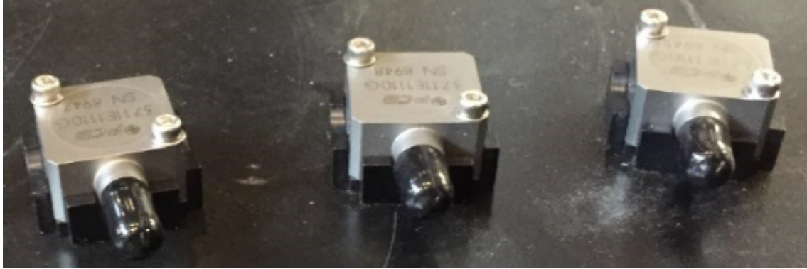
Fig. 3.5. 3711B110G accelerometers close-up.
