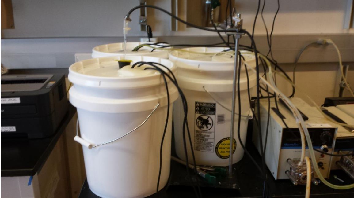
Figure 11: Photobioreactors. Photograph showing container, effluent/influent lines and pumps.
