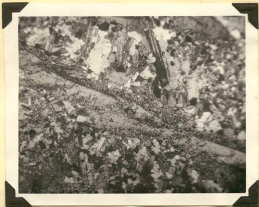
A. Photomicrograph of feather-like augite crystals in basic segregate (sample number OM-124).
