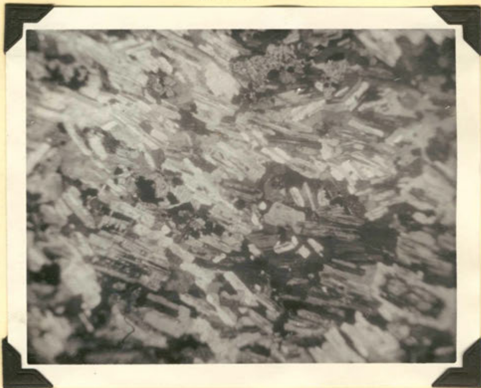
A. Photomicrograph of sub-parallel feldspar crystals demonstrating linear flow structure (sample number OM-265).
