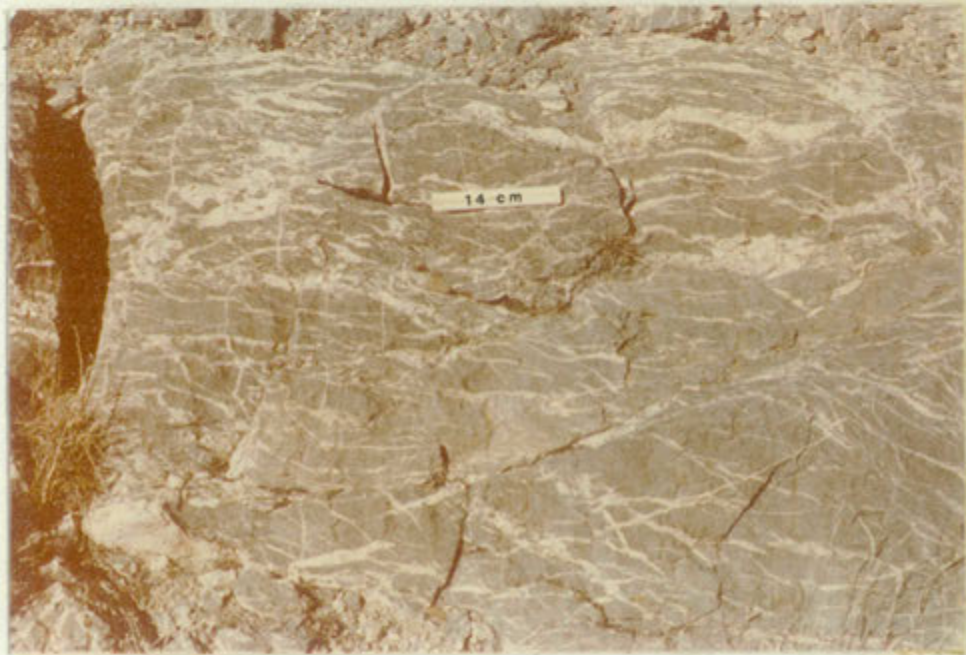
Figure 6. Echelon tension fractures filled with calcite veins in U-Bar Formation limestone underlying a klippe of Paleozoic limestone.
