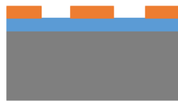
(b) Patterned and etched device layer
