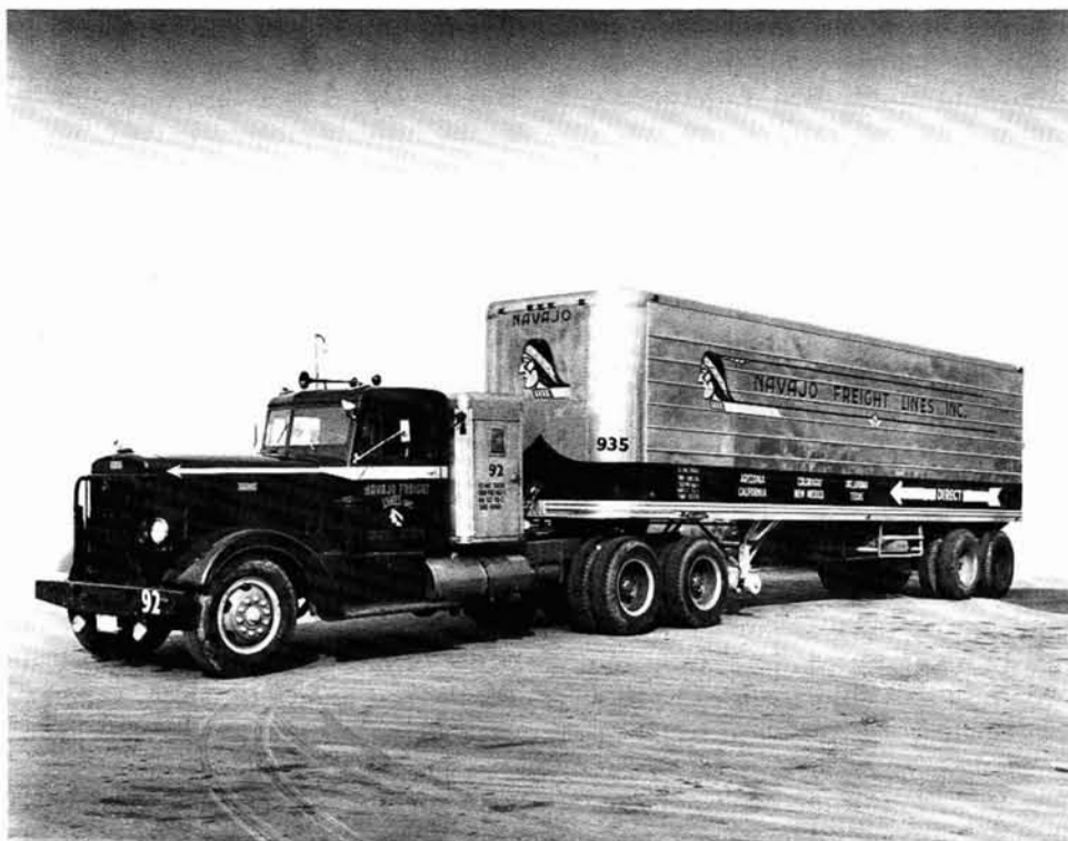
1952 Peterbilt conventional tractor with 35-foot Trailmobile trailer. Tractor had 6-cylinder "HB-600" Cummins Diesel, 672 CID giving 150 hp at 1800 rpm. Notice the sleeper is attached to the cab of the tractor. (Mitch Howe Collection)
