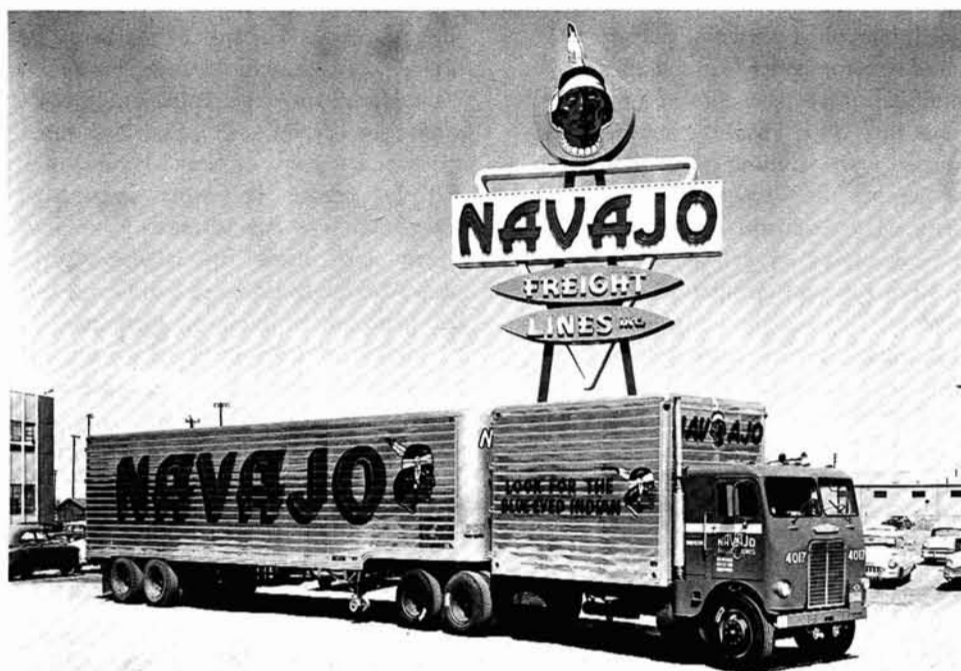
This is one of three 1964 White-Freightliner tractors with a dromedary trailer configuration. Notice the sleeper is now built into the cab. There were only three of these types of trucks built for Navajo Freight Lines. Photograph taken in front of the Denver Terminal. (Freightliner Corporation)
