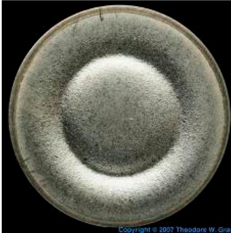
Figure 2.2 Sputtering target showing characteristic erosion pattern
