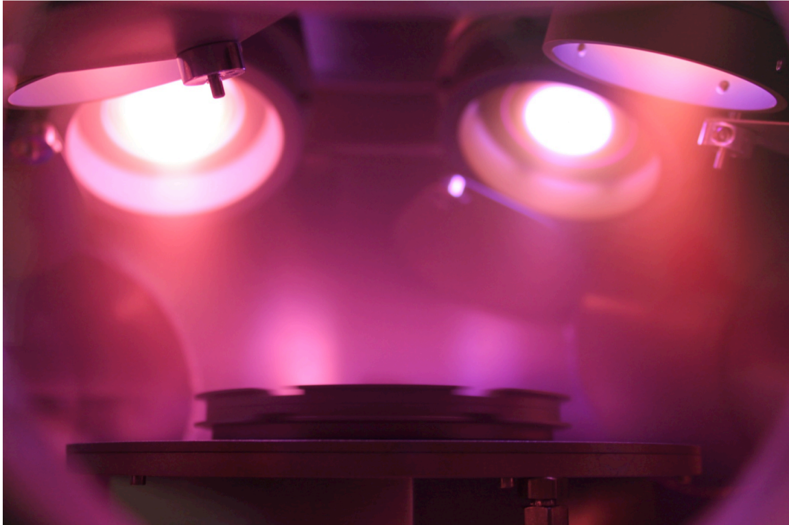
Figure 2.3 Inside of DC Magnetron Chamber (CINT Gateway Facility) showing plasma glow of four sputter guns with open shutters and rotating sample stage for even deposition.
