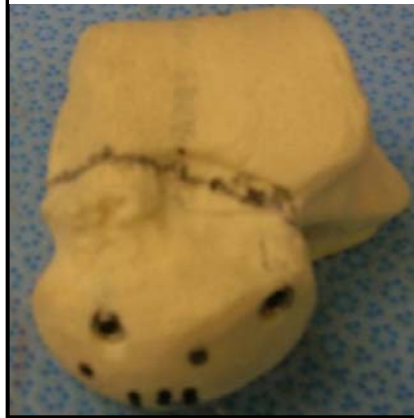
Figure 2: Fracture Through Talar Neck of Sawbone Specimen Fixed with CH Screw
