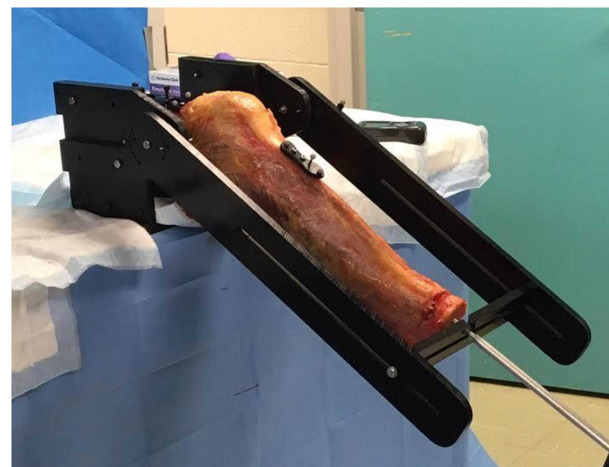
Figure 4: Side view of a cadaveric specimen fixed in the custom-made testing fixture at 30° of flexion with the torque/rod fixed in the distal tibial medullary canal
