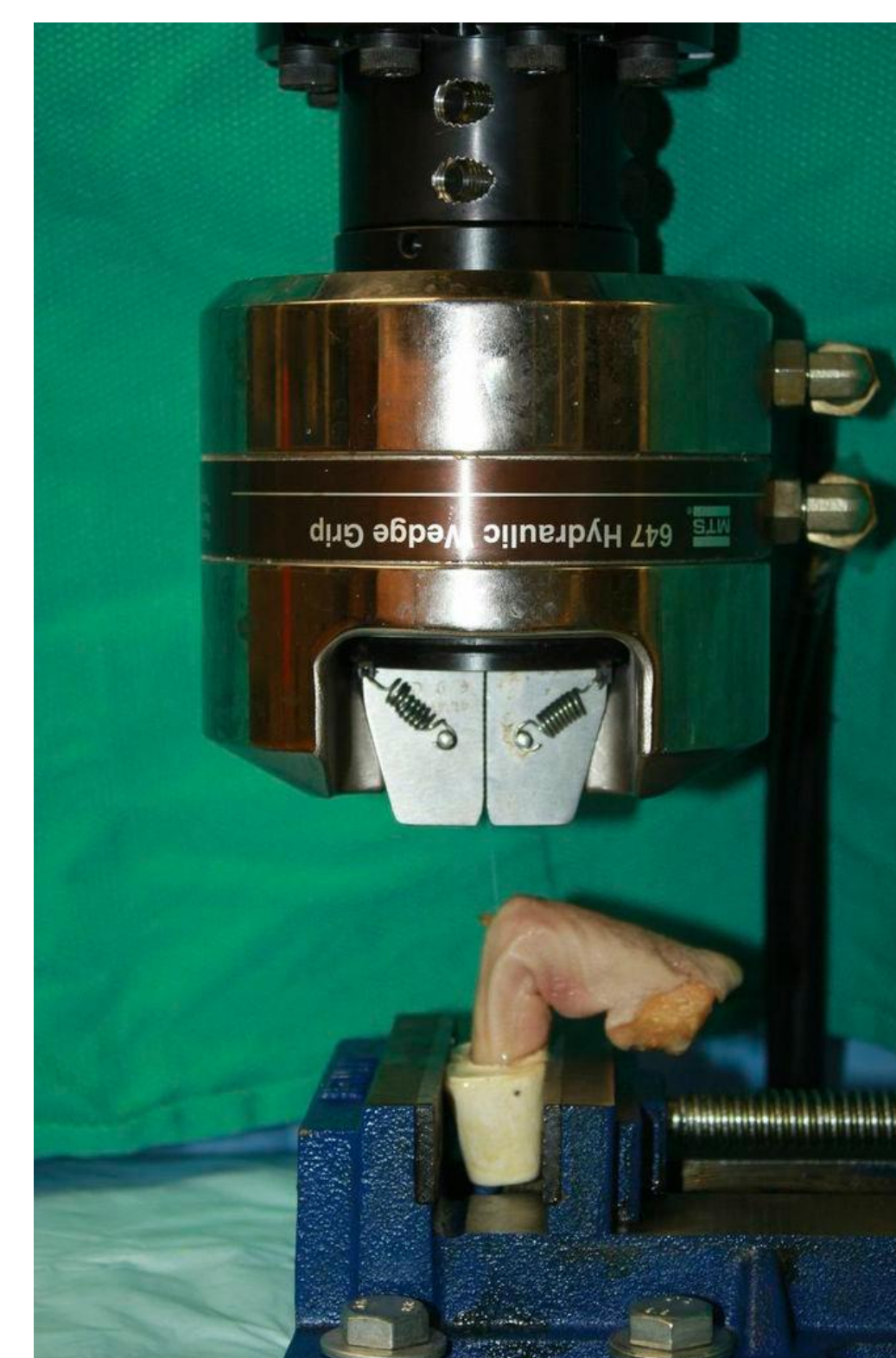
Figure 3: Experimental testing fixture showing specimen in bone cement fixed to the base of the testing machine. Suture attached to vertical actuator grips for tensile loading at a rate of 100mm/min.
