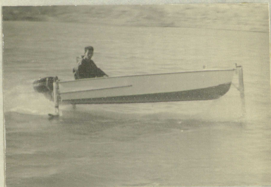
Figure 16.. Rough water jump takeoff with bar boosters in place.
