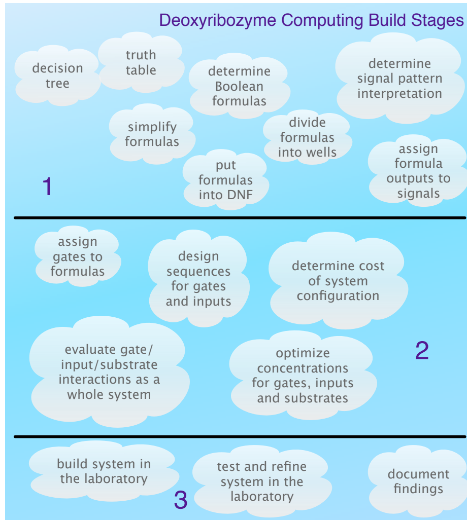
Figure 2.1: The current process for engineering a platform from concept to finished product can be divided into three stages, proceeding from top to bottom. These processes are deliberately shown disconnected, rather than in a flow chart, to reflect how the overall design and build engineering effort currently proceeds. There is no central, generally recognized, set of steps to program, build, and verify a deoxyribozyme computing platform.
