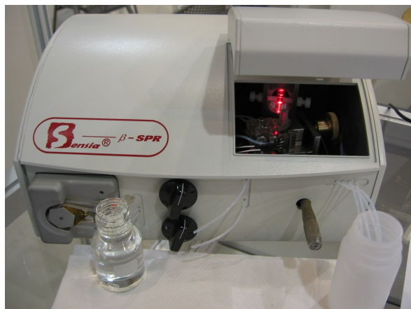
Fig. 2. Portable SPR platform, including sensor, optics, electronics and flow delivery system
