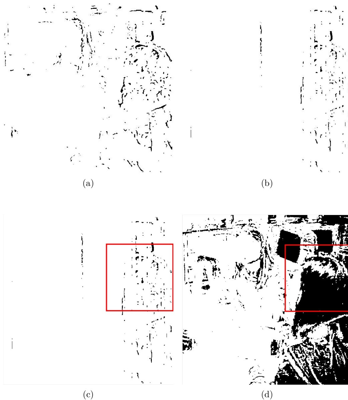
Figure 4.16: Back of the head detection: (a) Doing ‘AND’ operation between Fig. 4.15d and binary image of AM component. (b) 60 longest vertical lines. (c) The highest density area of black pixels. (d) Same area in AM component.
