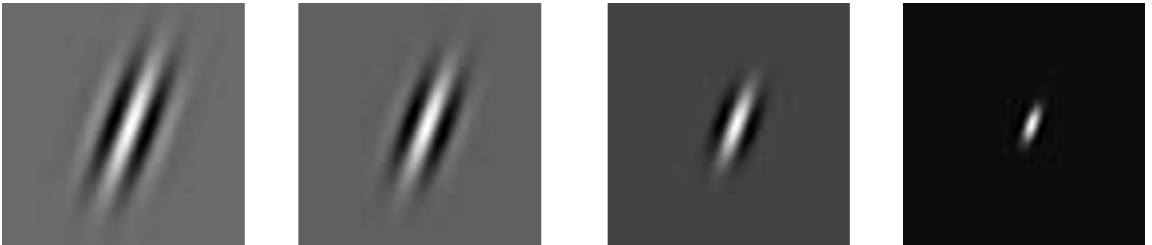
Figure 2.2: Gabor filter kernels with different sizes: \sigma=11, 9, 6 and 3 . Here, \text{Ang} = 20.25^\circ and F = 27/128 \cdot \pi .
