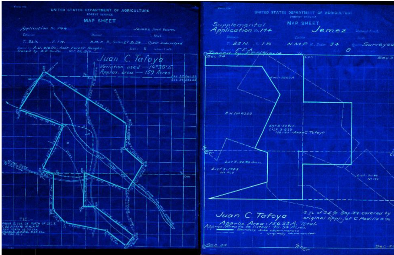
Figure 17: Map Sheet Form 220 for the homestead of Juan C. Tafoya, near Regina, NM. Left, a metes and bounds survey with seventeen angle points done in 1910. Right, the boundaries for Tafoya were redrawn in 1914 to solve conflict problems with neighboring homestead.
