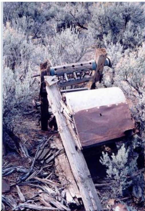
Figure 1 Left: A threshing machine for beans or triadora at the old homestead of Luis Trujillo (Photo courtesy of Chris Chávez c. 1998). Right: A hypothetical rendering of how the hand built machine may have operated (Illustration by Roberto H. Valdez).
