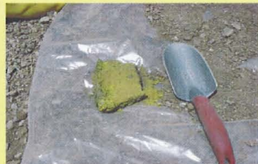
Photograph of depleted uranium removed from near the entrance to SWMU 28-2.
