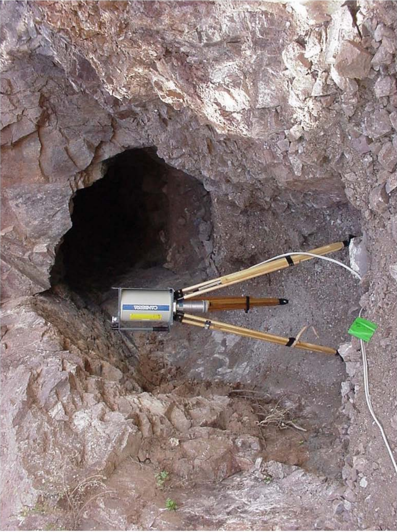
Figure 3.3-1. In situ soil gamma spectroscopy measurement at Solid Waste Management Unit 28-2
