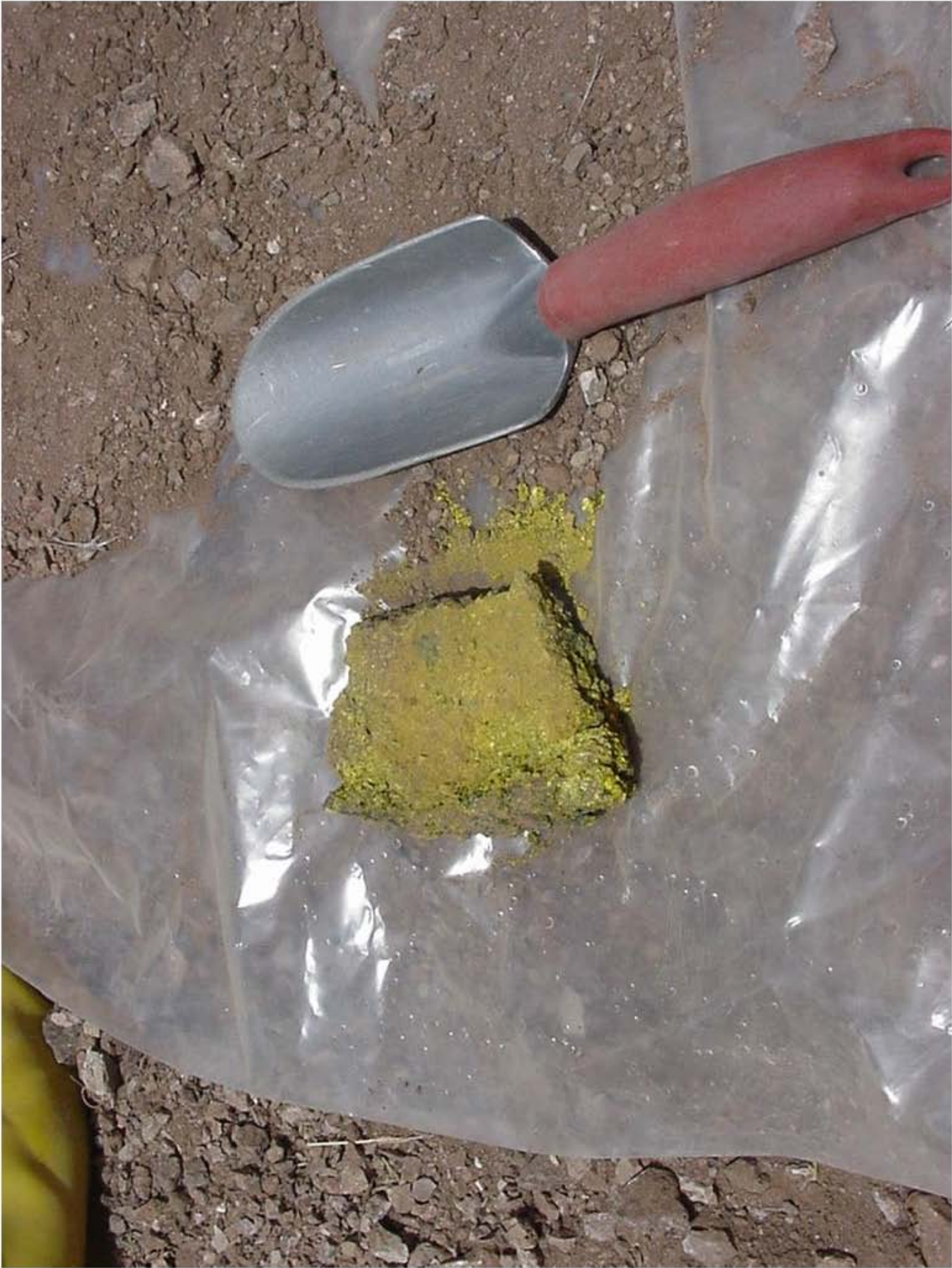
Figure 3.2-2. Depleted Uranium removed from the exterior at Solid Waste Management Unit 28-2
