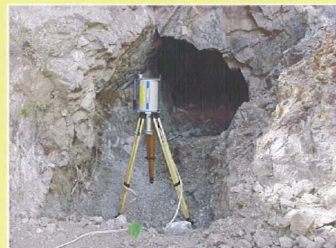
Photograph of in situ gamma spectroscopy measurement at SWMU 28-2
