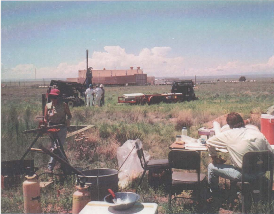
Figure 3.4-1 Collecting soil samples with the Geoprobe in the DSS Site 1033, Building 6631 septic system drainfield area. View to the west. August 16, 1999
