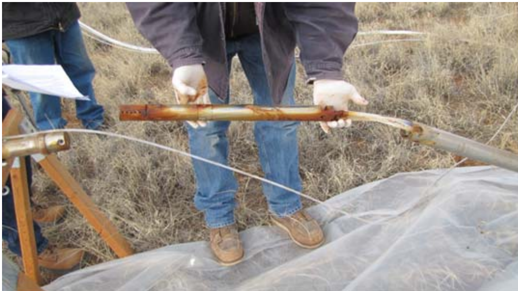
Figure 10-1 Photograph of Stainless Steel Sampling Pump Removed from Mixed Waste Landfill Groundwater Well MWL-MW4 on December 16, 2014
