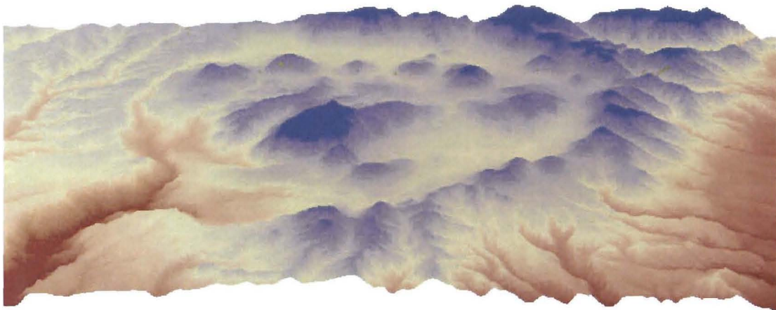
Figure 5: 3-dimensional topographic map of the Valles Caldera created by mosaic of 15' Quad Digital Elevation Models (DEMs) from http://rgis.unm.edu .
