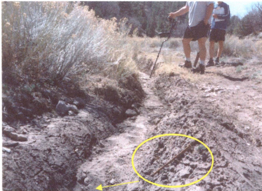
Figure 4-6 The metal detector in this picture shows the original location of Site 2A–pin 1. In April 2001, the pin was found 6m downstream of its original location and 0.4m in the ground.
