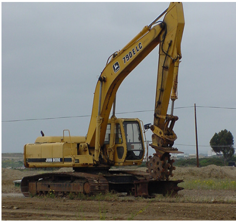
Figure 2. A sheep's foot roller can be used to “dimple” a slope as long as the action is not taken to an extreme, smooth and compacted surface. (Erosion Control Network)
