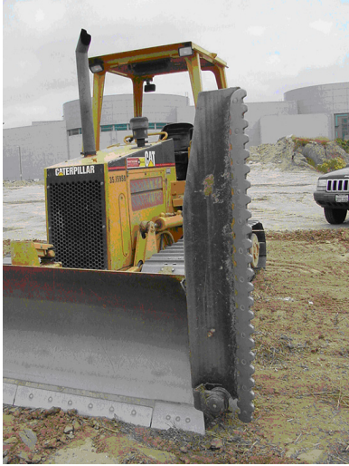
Figure 5. Slope boarding is generally applied to cut slopes and can provide and underlying structural support to hydraulic seed and mulching applications. (Erosion Control Network)
