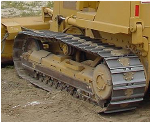
Figure 1. Grouser tracks on a bulldozer can be used as a surface roughening technique when the tracks go up and down a slope. However, if the tracks go across a slope, erosion is accelerated. (Erosion Control Network)
