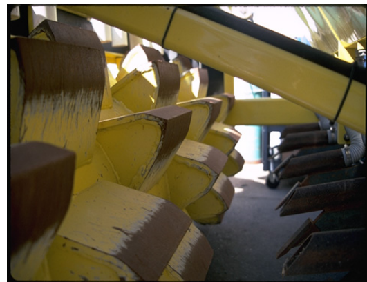
Figure 4. The resulting roughness created from imprinting creates an opportunity for water to and sediment to be collected and fosters the germination and growth of seed. (Erosion Control Network)
