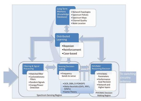
Figure 6: Proposed cognitive engine for a typical Radiobot.
