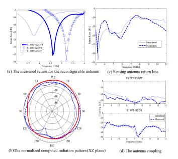
Figure 10: Performance of the combined sensing and cognitive communications reconfigurable antenna system.
