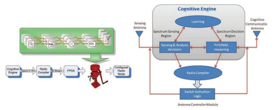
Figure 4: (a) Mix-n-match radio mode selections in a Radiobot system; (b) How Radiobot's CE controls its reconfigurable hardware through software-controlled switching circuits.
