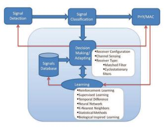
Figure 8: Inter-dependence of decision-making and learning inside the Radiobot's CE.
