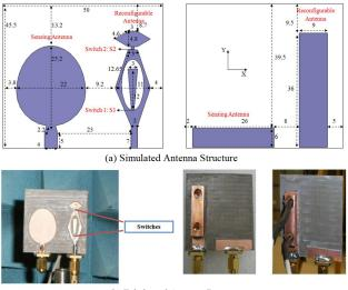
(b) Fabricated Antenna Prototype
