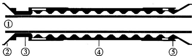
Fig. 4. Configuration of the uniform slow-wave structure. 1) Electron beam. 2) Anode of the *A-K* gap. 3) Cutoff neck. 4) Periodic ripple structure. 5) Impedance matching ring.
