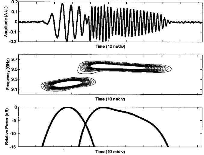
Fig. 9. Cross-excitation instability measured with a 10-period SWS. Top: Heterodyned frequency signal with a LO frequency of 9 GHz. Middle: SPVV time-frequency distribution. Bottom: Relative power in dB at the two mean frequencies of 9.21 and 9.57 GHz. ( $V_{\text{diode, pk}} = 350$  kV,  $I_{\text{b, avg}} = 1.2$  kA, and  $k_*L = 35.2$ .)
