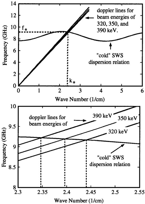
Fig. 1. The "cold" SWS dispersion relation of the UNM long pulse BWO at the  $TM_{01}$  mode. The resonant wavenumber  $k_*$  is defined by the intersection of the Doppler line with the cold SWS dispersion curve. (top) General overview. (bottom) Zoomed-in view of the SWS dispersion relation.
