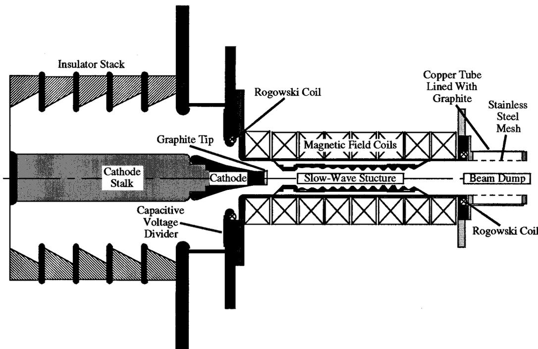
Fig. 3. Cross-sectional diagram of the long-pulse BWO.
