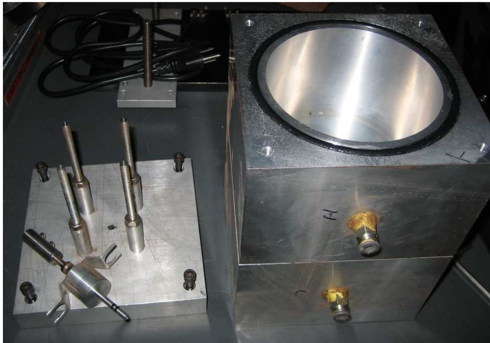
Figure 79. Pressure calibration chamber for \mu\text{BAR} . On the right are the stacked chambers, labeled “H” and “L”, with the top chamber opened to show the interior volume. The lid of the top chamber is on the left with the piston hole in the center and the piston sitting on top. The vertical posts on the lid are for mounting the stepper motor and the “wings” on the piston are guides to keep the piston from rotating.
