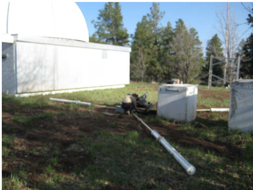
Figure 83. April 2008 \mu BAR setup with expansion chamber acoustic filters. The 1.0 meter telescope dome is to the left of the image.
