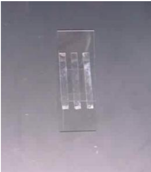
Figure 25: Two channel flow-cell for use in DNA tethering experiments.
