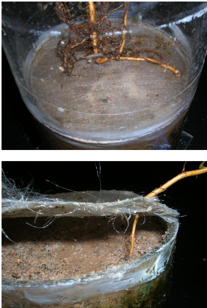
Figure 3.4 Photograph of root growth through geotextile
