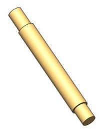
Figure 61: Separated Holder Neck for Variable Length
