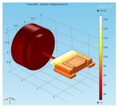
Figure 42: Temperature Distribution at 900 sec, Case 1, tBlock=0.75", LNeck =1.5"
