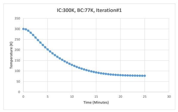
Figure 41: Cool Down Test, Case 1, tBlock=0.75", LNeck =1.5"
