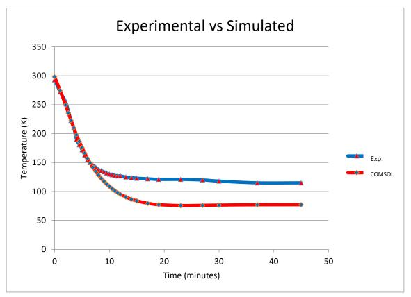
Figure 66: Temperature vs Time curve for Holder Cool Down
