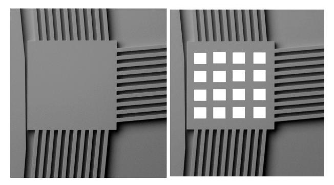
Figure 85: (Left) Present Chevron Junction (right) Improved Junction
