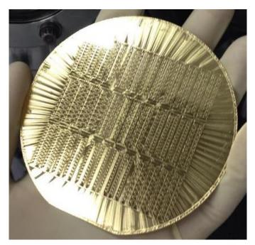
Figure 76: Sample Wafer Sputtered with Gold
