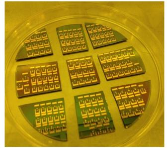
Figure 77: Diced Actuator Wafer
