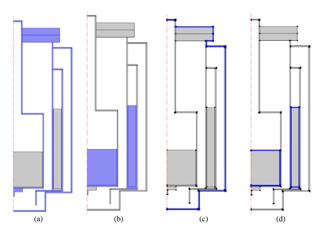
*Figure 8: Initial Conditions for case 1 a) 300K, b) 77K, Boundary Conditions for Case1 c) 10W/inch2, 300K inward Flux, d) 77K fixed temperature (Similar to figure 7)*
