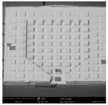
Figure 88: Gold Net (White) Stuck to BOX Layer Preventing Load Cell Motion
