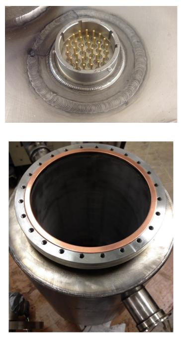
Figure 31: (Top) 32 Pin Connectors for Electrical Feedthrough (bottom) Copper Gasket for CF Flange
