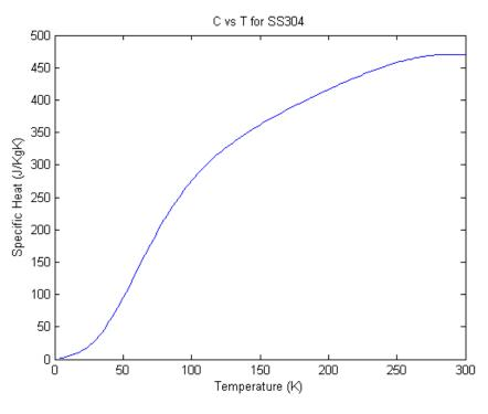
Figure 5: Heat Capacity for SS 304
