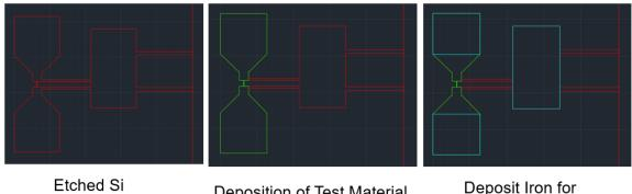
Deposition of Test Material e.g. Gold, Negative Photoresist PMMA etc. Deposit Iron for handling Sample through Magnetism
