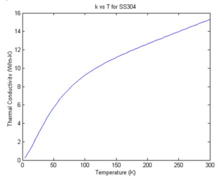
Figure 4: Thermal Conductivity of SS 304
