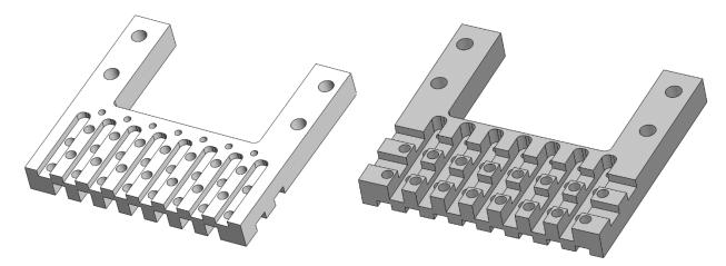
Figure 59: Ceramic Insulation for Electrical Connectors (Left) Top View, (Right) Bottom View
