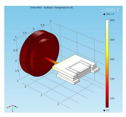
Figure 48: "Temperature Distribution, Heat Up Test, Case 1, tBlock=0.375", LNeck =1.4"
