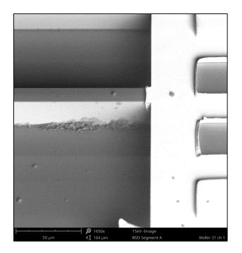
Figure 87: Residue Preventing Load Cell Motion
