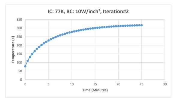
Figure 49: Heat Up Test, Case 1, tBlock=0.375", LNeck =1.4
