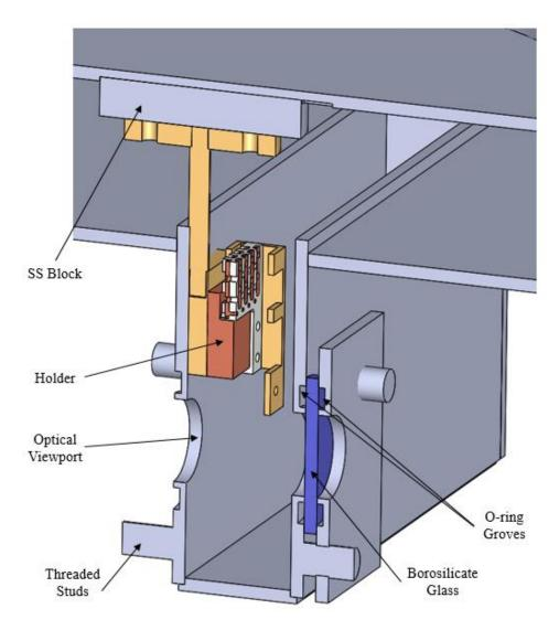
Figure 29: Optical Access for Cryostat
