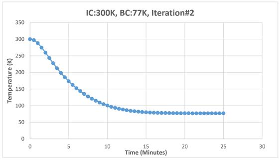
*Figure 44: Cool Down Test, Case 1, tBlock=0.75", LNeck =1"*
