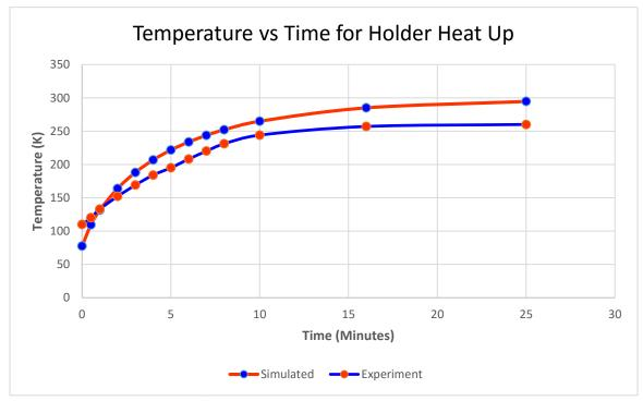
Figure 67: Temperature vs Time curve for Holder Heat Up
