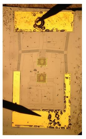
Figure 84: Thermal Actuator with Probe Needle
