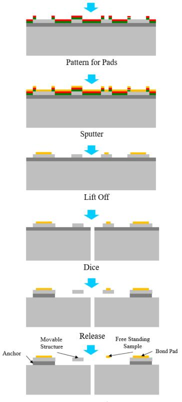
XeF<sub>2</sub> Etch Figure 79: Fabrication Process Flow
