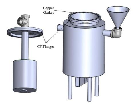
Figure 28: Separable Parts for the Cryostat
