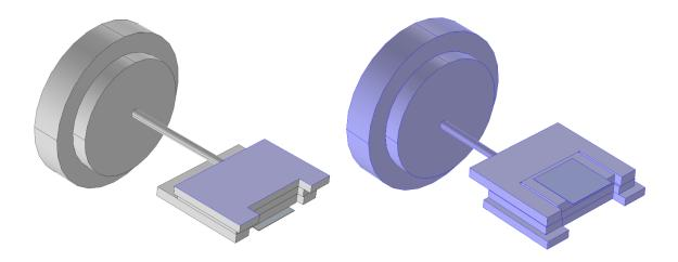
Figure 54: (Left) 10 W/inch2 Boundary Condition (Right) 4.5K Initial Condition for Heat Up Test, Case 2
