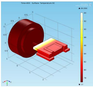
*Figure 43: Temperature Distribution at 900 sec, Case 1, tBlock=0.75", LNeck =1"*
