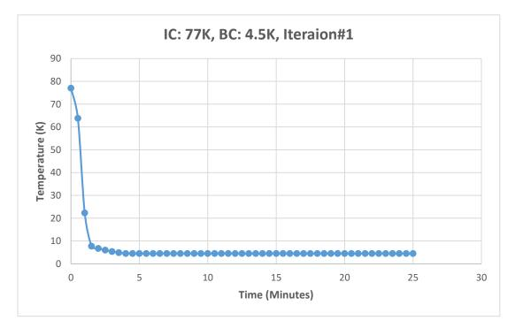
Figure 52: Cool Down Test, Case 2, tBlock=0.375", LNeck =1.4"
