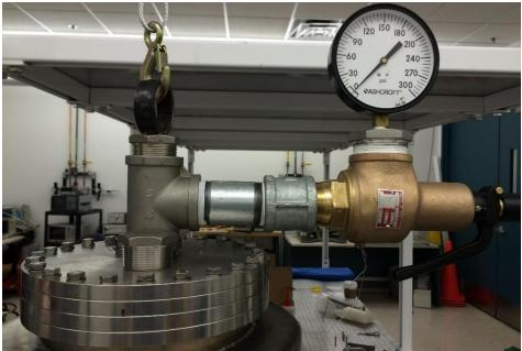
Figure 32: Relief Valves (150 psi) added to the Inner and Outer Chamber Inlets
