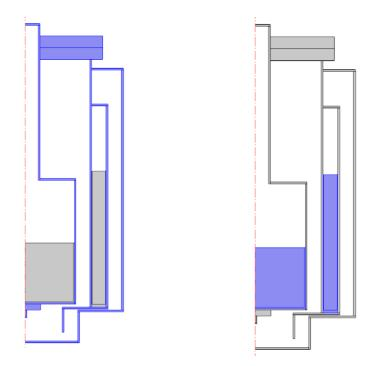
Figure 6: Highlighted Areas show Material Assignment for SS 304 (Left) and Liquid Nitrogen (Right) for Case 1
