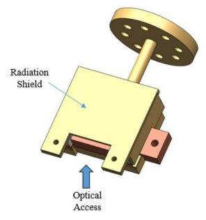
Figure 60: Protective Cover for Sample
