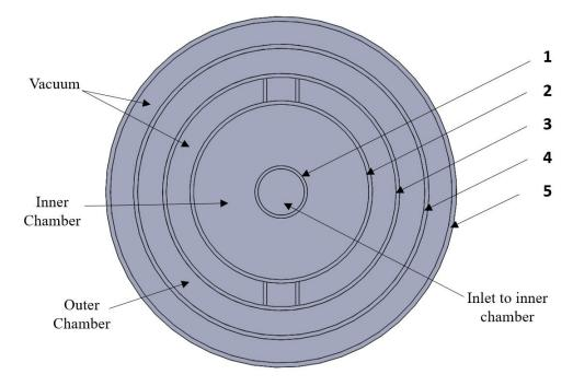
Figure 1: Cross Section of Cryostat
