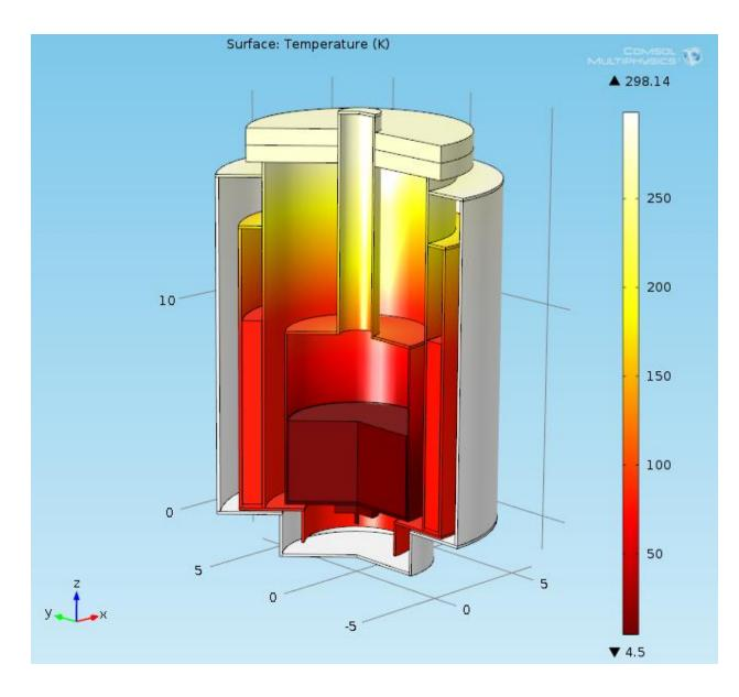
Figure 25: A steady State Analysis Showing the Temperature of Cryostat for Case-2
