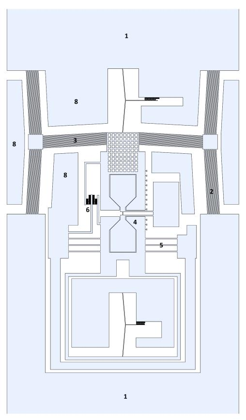
Figure 68: Cascaded Thermal Actuators with Interchangeable Sample
