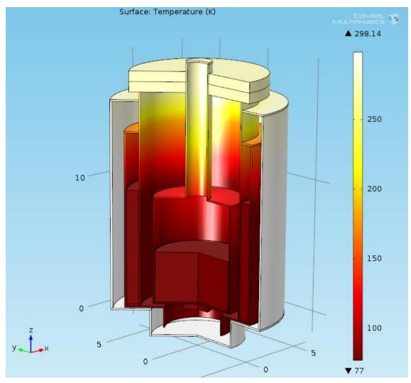
Figure 20: A steady State Analysis Showing the Temperature of Cryostat for Case-1
