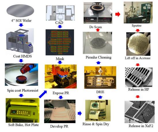
Figure 78: Summarization of Fabrication Process.
