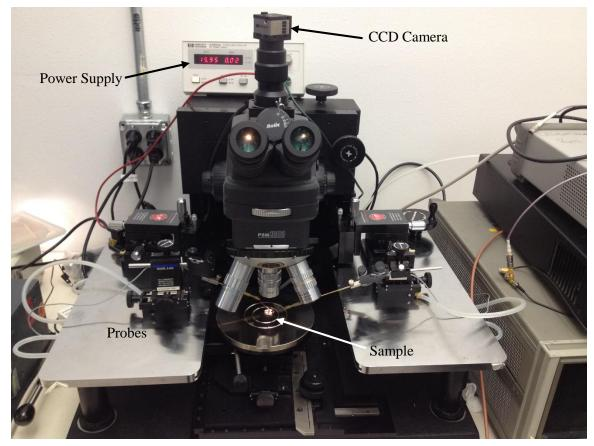
Figure 82: Experimental Setup for Thermal Actuators
