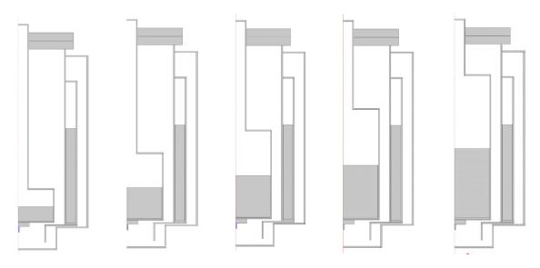
*Figure 13:: Design Iterations for Inner Chamber Length (Left to Right: L=r, 2r, 2.5r, 3r, 4r)* The relative performance of each design iteration is observed by comparing the consumption rate at 15 minutes (Start of quasi steady state, converted to per hour) vs. the capacity of the inner chamber.
