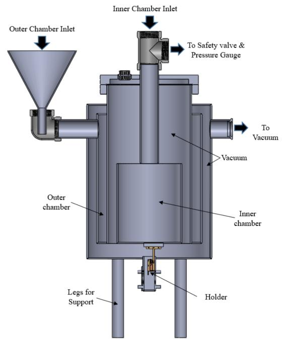
Figure 27: Cross Sectional View of Cryostat
