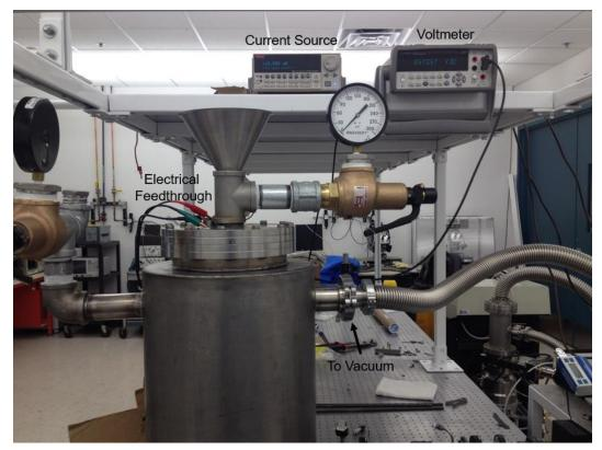
Figure 34: Experimental Setup for Testing of Cryostat
