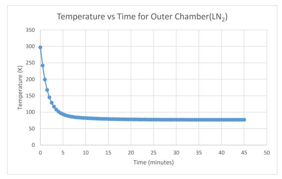
Figure 19: Temperature vs Time for Outer Chamber – Case 1
