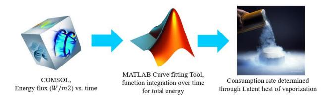
Figure 10: Steps Involved in Calculation of Consumption Rates for Cryogenic Liquids
