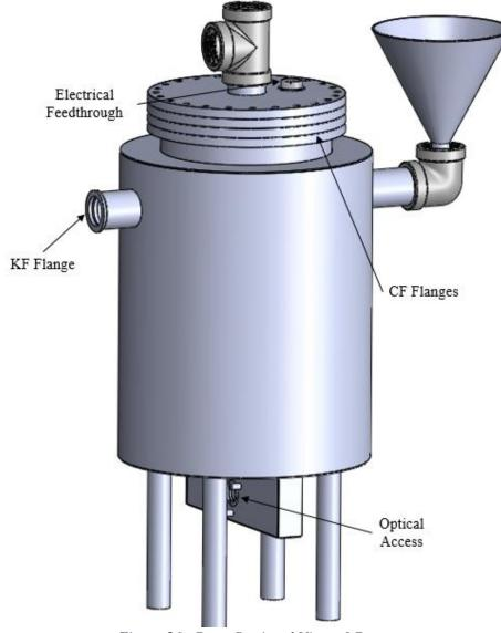
Figure 26: Cross Sectional View of Cryostat
