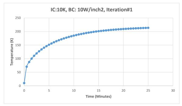
Figure 55: Heat Up Test, Case 2, tBlock=0.375", LNeck =1.4"
