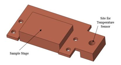
Figure 58: Copper Sample Stage
