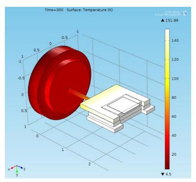
Figure 56: Temperature Distribution, Heat Up Test, Case 2, tBlock=0.375", LNeck =1.4"
