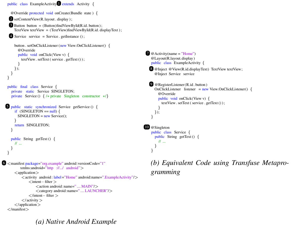
Figure 1.1: A simple Android example compared with an equivalent application outfitted with transfuse. This example shows a 33:18 reduction in the amount of hand written code.
