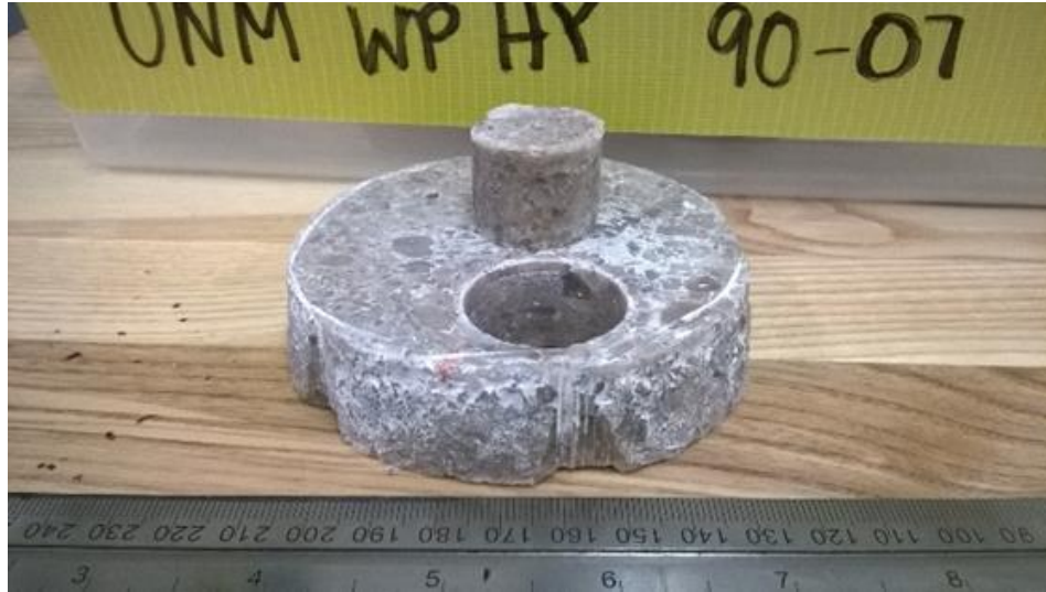
Figure 2 A 25.4 mm diameter core obtained from 100 mm in diameter and 25 mm thick disc.
