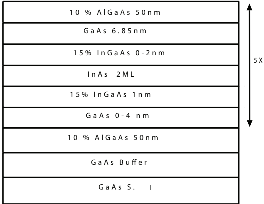
Figure 2.1: Baseline structure used for optimizing DWELL detectors. The GaAs layer under the dot and the \text{In}_{0.15}\text{Ga}_{0.85}\text{As} capping layer above the dot were optimized using this structure.
