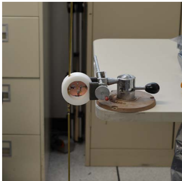
Figure 26. Photograph of the active dipole antenna.
