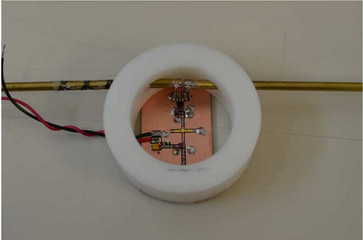
Figure 24. Photograph of the prototype active dipole installed in the prototype housing.
