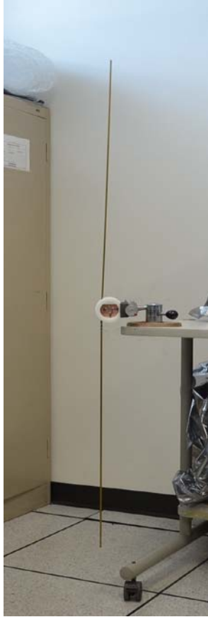
Figure 25. Photograph of the full size prototype active dipole antenna.
