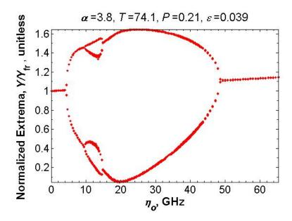
Figure 66. Theoretical simulation of the quantum-dash laser's dynamic response at 85 mA and zero-detuning.
