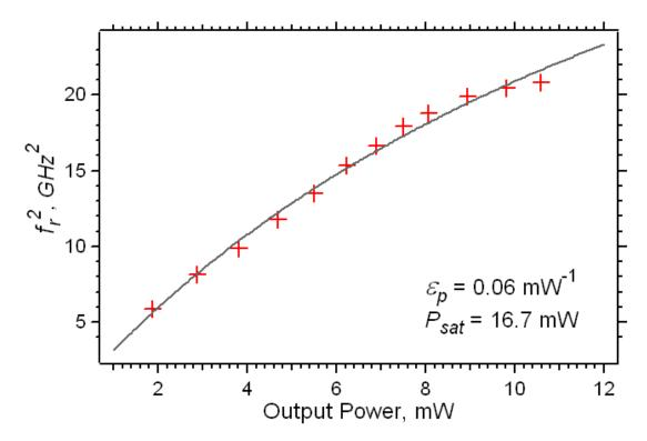
Figure 48. Quantum-dot laser free-running relaxation oscillation  $(f_{fr}^2)$  as a function of the total output power ( $P_{out}$ , both laser facets). The dotted line is a least squares linear fit using expression (93).
