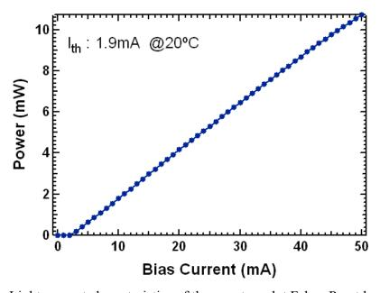
Figure 34. Light-current characteristics of the quantum-dot Fabry-Perot laser showing a measured threshold current of 1.9 mA at 20°C.
