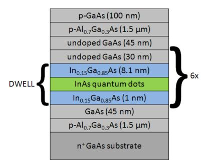
Figure 33. Epitaxial layer composition of the quantum-dots-in-a-well laser structure.
