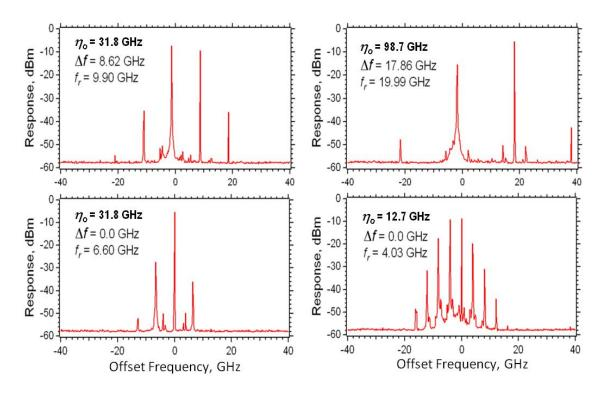
Figure 67. Optical spectra of the optically-injected quantum-dash slave biased at 65mA.
