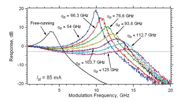
Figure 58. Normalized microwave modulation response under zero-detuning for increased injection strengths; slave bias is 85 mA.
