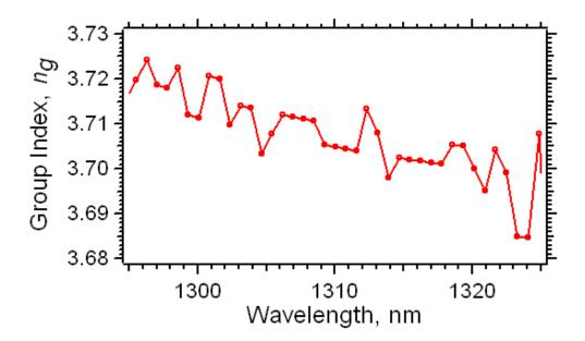
Figure 36. Group index of the active region as a function of Fabry-Perot mode at a bias current of 5 mA. The free-spectral range  $(\Delta \lambda)$  was averaged between each two adjacent modes, and calculated using  $n_g = \lambda^2/(2L\Delta\lambda)$ .
