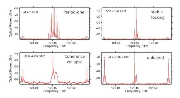
Figure 64. Negative frequency detuning series for a maximum injection strength of 14.2 GHz and a slave laser bias of 65 mA.
