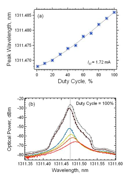
Figure 40. Quantum-dot laser: (a) Peak modal wavelength as a function of duty cycle. The pulse width was 20µs. (b) Optical power response for subthreshold bias currents at 100% duty cycle. The bias currents correspond to 1.1 mA (red), 1.3 mA, 1.5 mA, 1.7 mA, 1.9 mA, and 2.0 mA (gray).
