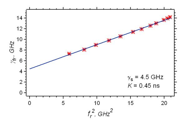
Figure 47. Free-running damping rate  $(\gamma_{fr})$  as a function of the relaxation oscillation frequency squared  $(f_{fr})^2$ . The blue line is a least squares linear fit to the data points, which is then extrapolated to determine the spontaneous carrier relaxation rate,  $\gamma_s$ .
