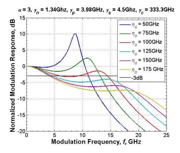
Figure 18. Modulation response as a function of maximum injection strength at zero-detuning,  $\alpha = 3$ . The free-running laser parameters are based on the quantum-dash laser biased at 70 mA.
