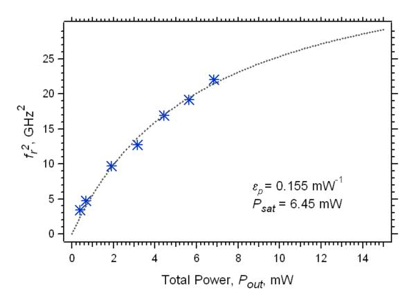
Figure 39. Quantum-dot laser free-running relaxation oscillation  $(f_{fr}^2)$  as a function of the total output power  $(P_{out})$ . The dotted line is a least squares linear fit using expression (93), where the gain compression coefficient is found to be 0.155 mW<sup>-1</sup>. In each plot, the experimental values (blue asterisks) correspond to laser bias currents of 3.8, 5, 10, 15, 20, 25, and 30 mA.
