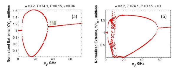
Figure 30. Bifurcation diagrams predicting the stability at zero-detuning where the nonlinear carrier relaxation rate parameter is (a) and is not considered (b) in the normalized rate equations.
