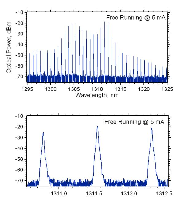
Figure 35. Optical spectra of the free-running quantum-dot laser observed under a bias current of 5mA. Top: 30-nm span. Bottom: 2-nm span.
