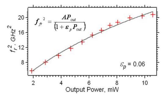
Figure 24. (top) Illustration of free-running nonlinear carrier relaxation rate and differential carrier relaxation rate saturation with increased laser output power. (bottom) Saturation of the relaxation oscillation frequency squared with increased laser output power. Data shown was collected on the quantum-dash Fabry Perot laser.
