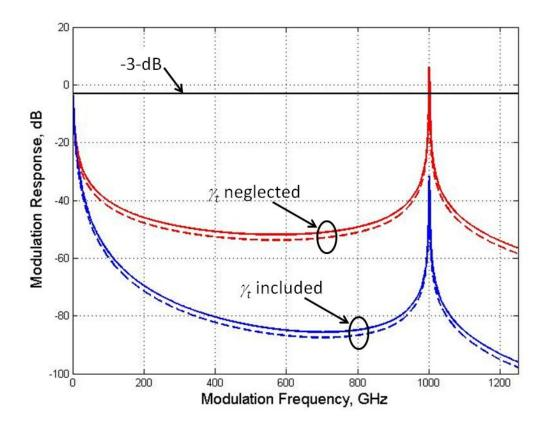
Figure 53. Theoretically simulated small-signal modulation response at the positive frequency detuning edge for a short cavity device (25  $\mu$ m) under strong injection ( $P_{inj}$  = 87.5 mW) to show a 1 THz resonance frequency. Cases where the inverse parasitic carrier transport time ( $\gamma_i$ ) is and is not considered are included. The dashed lines illustrate the impact of gain compression on the response.
