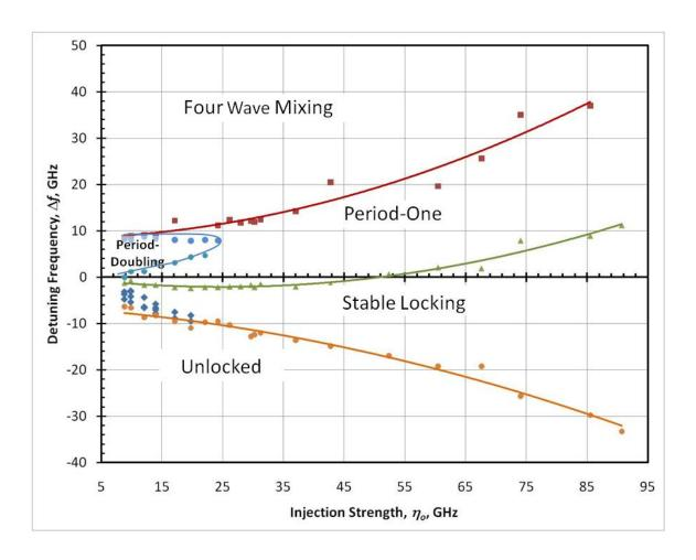
Figure 62. Stability map for the optically-injected quantum-dash slave laser at a bias current of 85 mA. The blue diamonds at negative detuning indicate chaotic (coherence collapse) operation. The trendlines have been added as a visual aid only.
