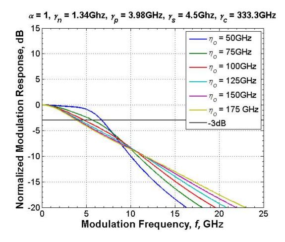
Figure 19. Modulation response as a function of maximum injection strength at zero-detuning,  $\alpha = 1$ . Compared with Figure 18, the response is more strongly damped. The free-running laser parameters are based on the quantum-dash laser biased at 70 mA.
