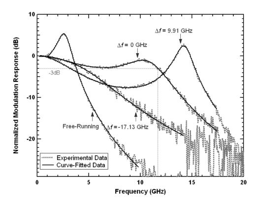
Figure 3. Modulation response of the injection-locked quantum-dash laser for varied frequency detuning ( $\Delta f$ ) conditions.
