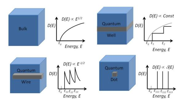
Figure 8. Cartoon of the basic structure and the associated density of states of bulk, quantum-well, quantum-wire, and quantum-dot semiconductor material.
