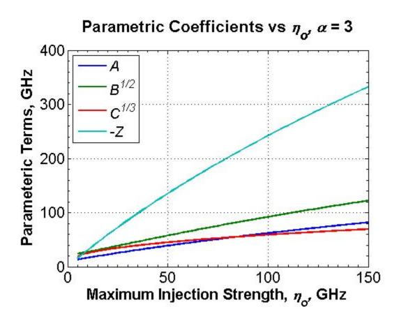
Figure 20. A, B, and C coefficients as a function maximum injection strength at zero-detuning,  $\alpha = 3$ . Notice that the resonance frequency driving term,  $B^{1/2}$ , remains larger than the damping rate driving term, A. The free-running laser parameters are based on the quantum-dash laser biased at 70 mA ( $\gamma_n = 1.34$  GHz,  $\gamma_p = 3.98$  GHz,  $\gamma_s = 4.5$  GHz,  $\gamma_c = 333.3$  GHz).
