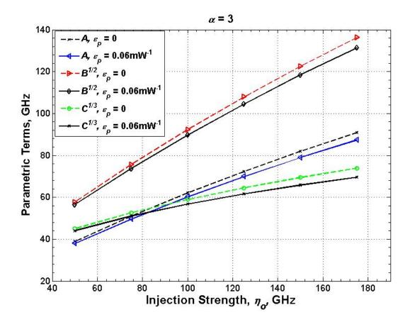
Figure 26. A, B, and C parametric terms plotted both with and without the consideration of the gain compression effect on the differential and nonlinear carrier relation rates plotted as a function of maximum injection strength at zero-detuning;  $\alpha = 3$ . The free-running laser parameters are based on the quantum-dash laser biased at 70 mA, and the gain compression coefficient is 0.06 mW<sup>-1</sup>.
