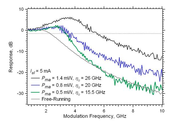
Figure 77. Normalized small-signal modulation response at zero-detuning.
