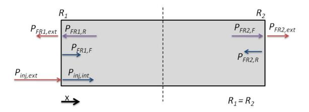
Figure 12. Illustration of the approach taken to calculate the external to internal injected power ratio where the output at both slave laser emitting facets is considered. The internal power ratio is taken at the center of the slave laser cavity, indicated by the dotted line. The internal power ratio is given by:  $R_{int} = P_{inj,int}/(P_{FRI,F} + P_{FR2,R})$ .
