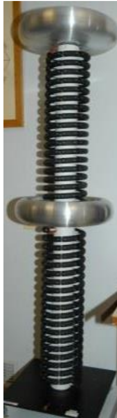
Figure 1.3.1. A two stack 200 kV DC divider developed at Australia's NMI. There are approximately 150 thin film resistors chained together helically for each divider stack. Individual resistors are encased in metallic tubing and the entire chain wraps around an insulating tube. Each divider stack has a nominal resistance of 220 M \Omega . This photo was taken in the DC Electrical Lab at the PSL.
