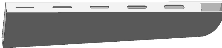
Figure 6.1: Modified narrow-wall longitudinal-slot array for higher gain.
