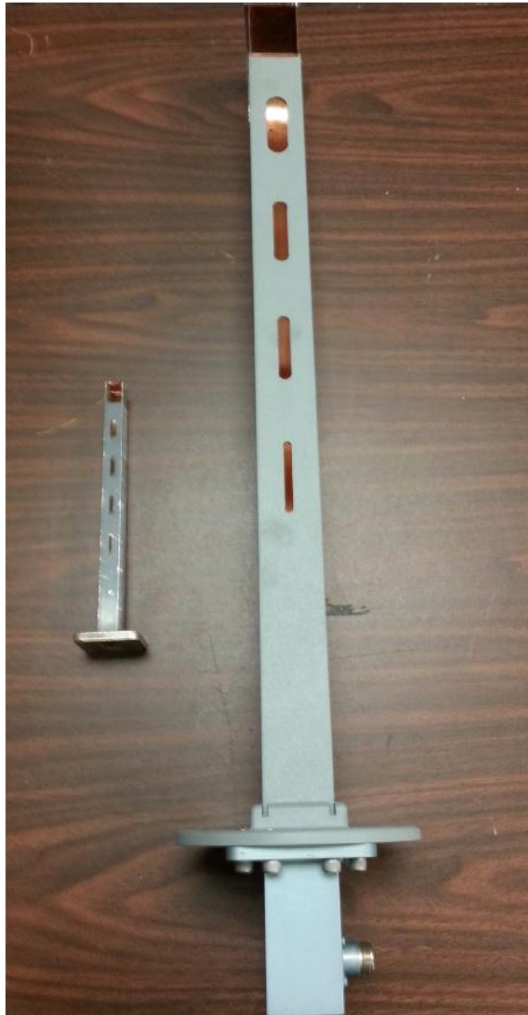
Figure 5.1: the S-band narrow-wall longitudinal-slot array (right) aligned with the X-band narrow-wall longitudinal-slot array (left).
