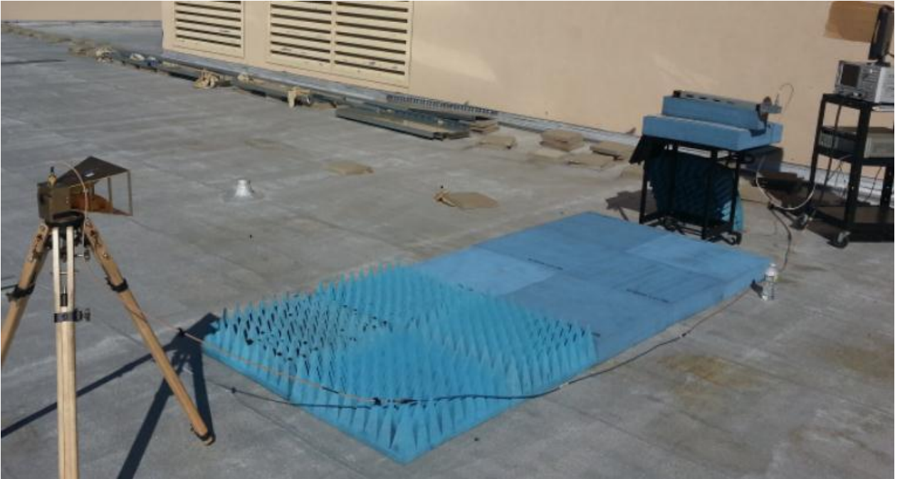
Figure 5.6: Overview of the experimental set-up for measuring the H-plane radiation pattern of S-band narrow-wall longitudinal-slot array antenna.
