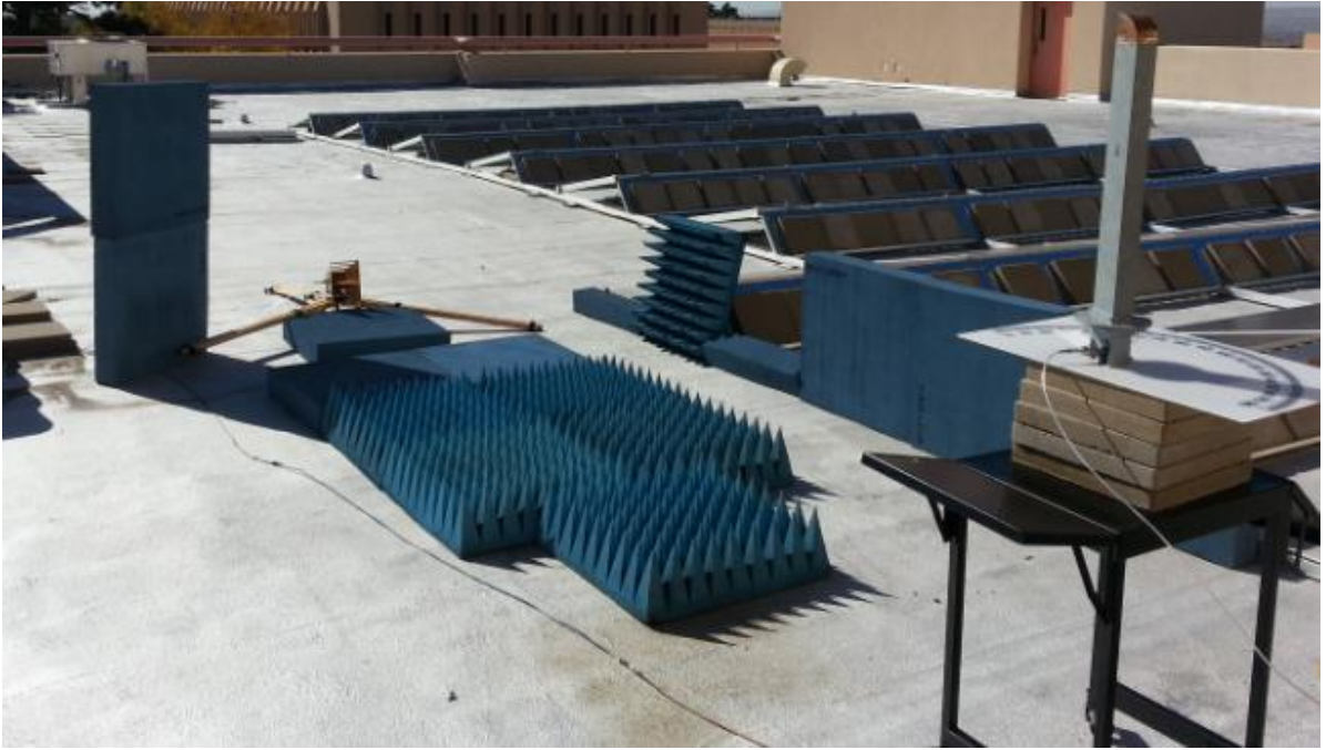
Figure 5.7: Experimental set-up for measuring the plane cut that is orthogonal to the H-plane and passing through the \theta = -15^\circ line shown in Figure 5.8 radiation pattern of S-band narrow-wall longitudinal-slot array antenna.
