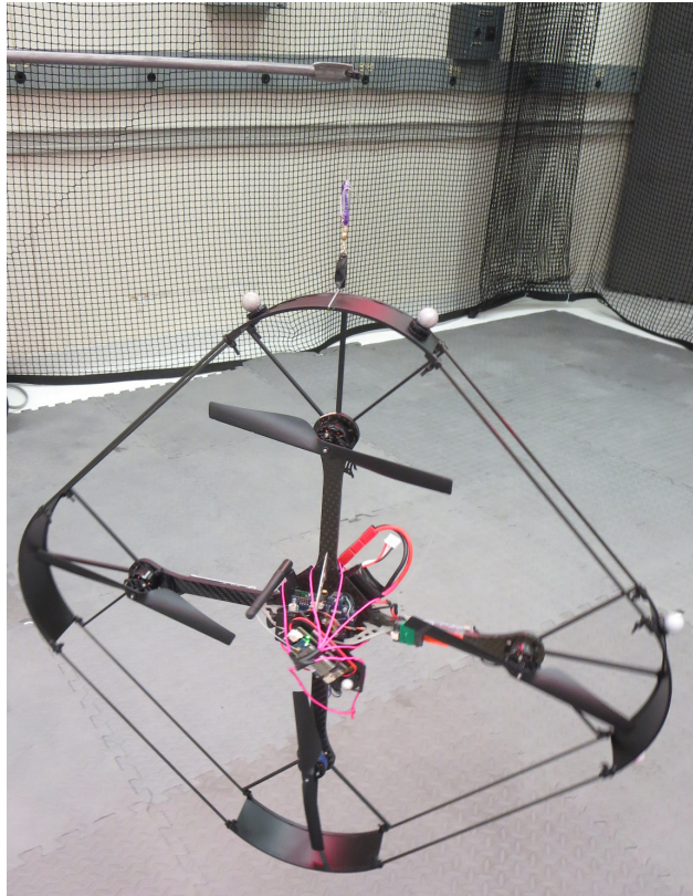
Figure 11.6: Picture of the suspended quadrotor while testing its pitch rotational inertia.
