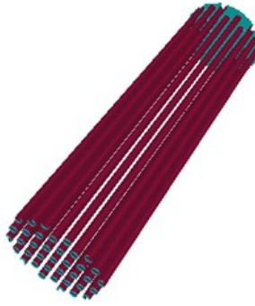
Figure 3.2.49. Schematic of a rodded cathode.
