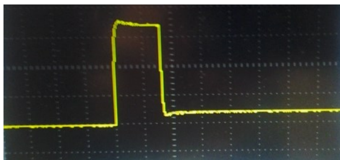
Figure 4.1.7. Current waveform for the UNM thyristor trigger circuit.
