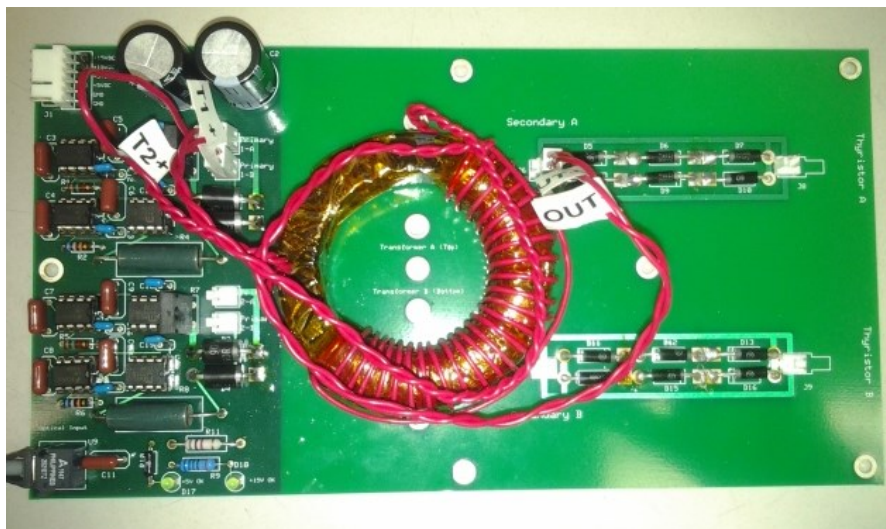
Figure 4.1.6. UNM's thyristor trigger circuit.
