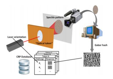
Fig. 2.2: Basic operation of an optical PUF [12].
