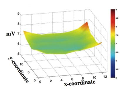
Fig. 3.4:  $V_{DD}$  profile using SMCs of a 90 nm chip.
