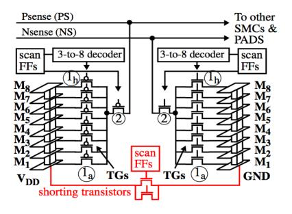
Fig. 4.1: SMC schematic in 90 nm chips.
