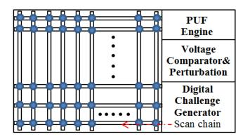
Fig. 5.2: PUF IP-block (blue circles represent SMC arrays).
