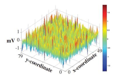
Fig. 3.5: Voltage drops from 4,000 SMCs on a PG65 chip.
