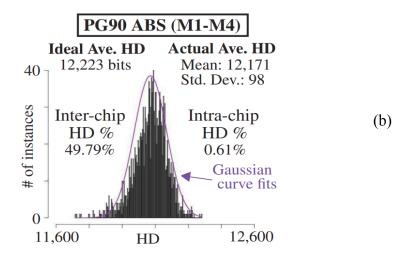
Fig. 3.7: Distribution of HDs using (a) stable DIFF (M1-M4) (b) stable ABS (M1-M4) bit strings from PG90 exps.
