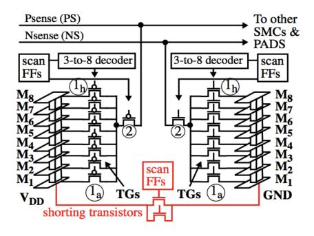
Fig. 3.2: SMC schematic in 90 nm chips.
