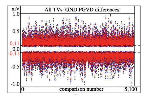
Fig. 4.3: CHIP<sub>1</sub> GND PGVD differences computed for bit generation during enrollment (a) and regeneration (b) at 9 TVs. Points in upper portion of plots generate '1's, points in lower portion generate '0's.
