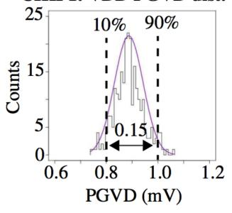
Fig. 4.2: CHIP<sub>1</sub> GND and  $V_{DD}$  PGVD distribution with Gaussian curve fits and 10% and 90% thresholds.
