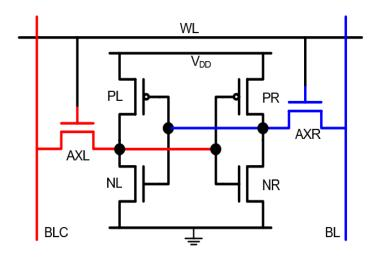
Fig. 2.6: Six transistor SRAM cell [29].
