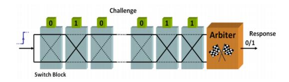
Fig. 2.3: Basic operation of an arbiter PUF [12]
