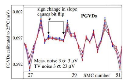
Fig. 4.10: Subset of PGERD (top) and PGVDs (bottom) from M2-M3 metal layer pairing for GND grid. Data from 9 TV corners is calibrated to 25°C, 1.2V. All 11 samples from 9 TV corners are also shown for each SMC.
