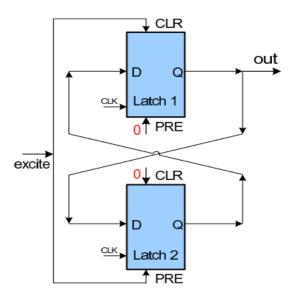
Fig. 2.7: Butterfly PUF: cross-coupled latches [32].
