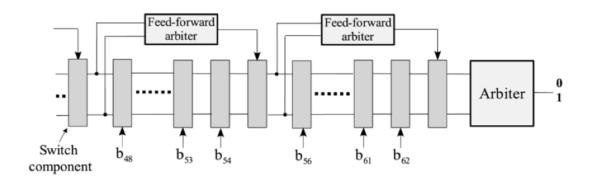
Fig. 2.4: Feed-forward arbiter scheme for improved security [19].
