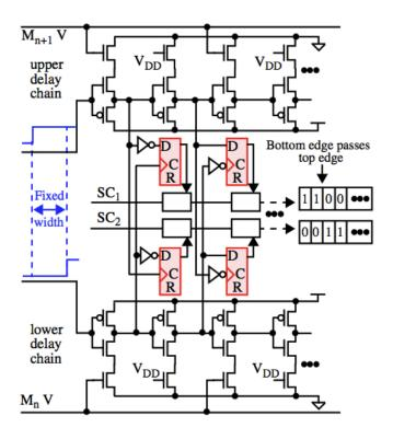
Fig. 5.1: Proposed differential-Power-Analysis (DPA) resistance VDC.
