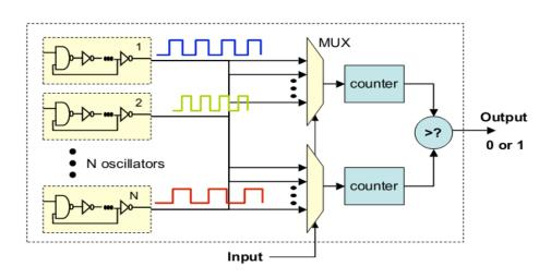
Fig. 2.5: Basic Ring-Oscillator PUF circuit proposes in [7].
