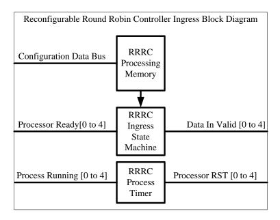
Figure 12. RRRC Ingress Block Diagram
