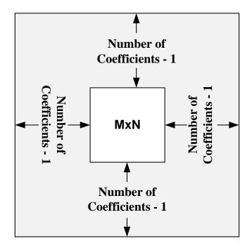
Figure 22. Filter Memory Structure.
