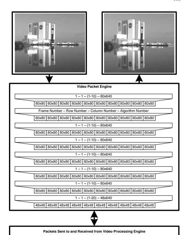
Figure 25. Packet Identification Process
