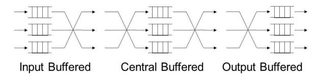
Figure 4. Switch Buffer Architectures [41]
