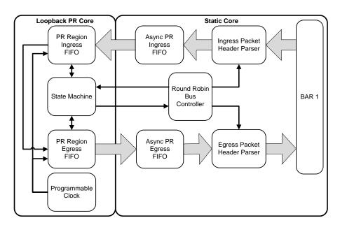
Figure 19. L-DPR-STM Core Block Diagram
