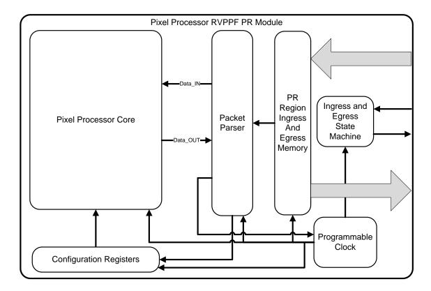
Figure 28. Pixel Processor PR Module
