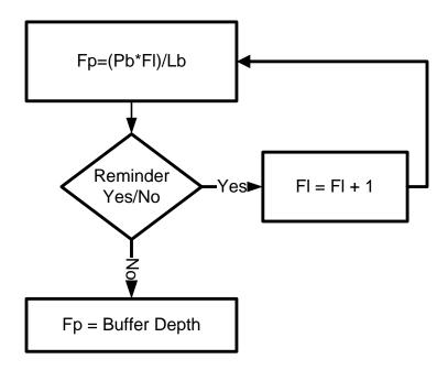
Figure 24. Buffer Depth Process
