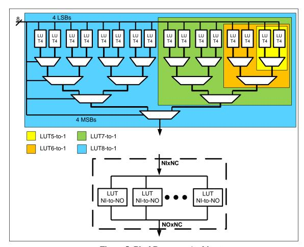
**Figure 5: Pixel Processor Architecture**
