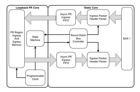
Figure 20. L-DPR-CTM Core Block Diagram
