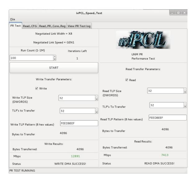
Figure 18. Speed Test GUI
