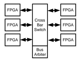
Figure 2. Splash 2 Interconnection Architecture
