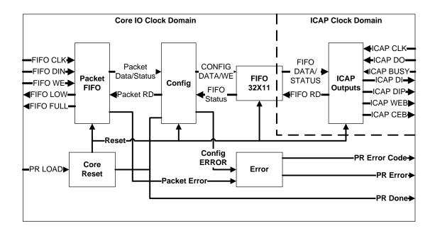
Figure 14. DPR Packet FIFO
